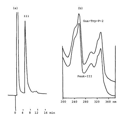
Column: Polygosil  ${}_5C_{18}$ , 4.6ø x 150 mm Solvent:  $CH_3OH(45\$)-H_2$ ) (54%)- $NH_4OHaq.(1\$)$
