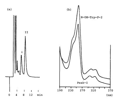
Column: Polygosil  ${}_5{}^{\rm C}_{18}$ , 4,6ø x 150 mm Solvent: CH ${}_3{\rm CN}$ (40%)-0.02 M KH ${}_2{\rm PO}_4$ (60%)
